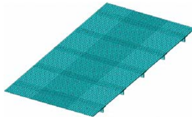
Figure 1. FE model of the stiffened composite panel analysed.
